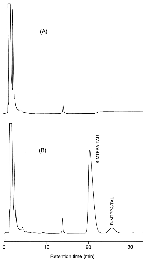
Fig. 3. Chromatograms of R,S -MTPPA-TAU. (A) Blank dog urine, (B) 24-h dog urine sample after administration of R -MTPPA at the dose of 10 mg/kg. S - and R -MTPPA-TAU in (B) were estimated 131.5 and 10.4 µg/ml, respectively. The absorbance unit (full scale=0.08 AU) was employed at 272 nm.
